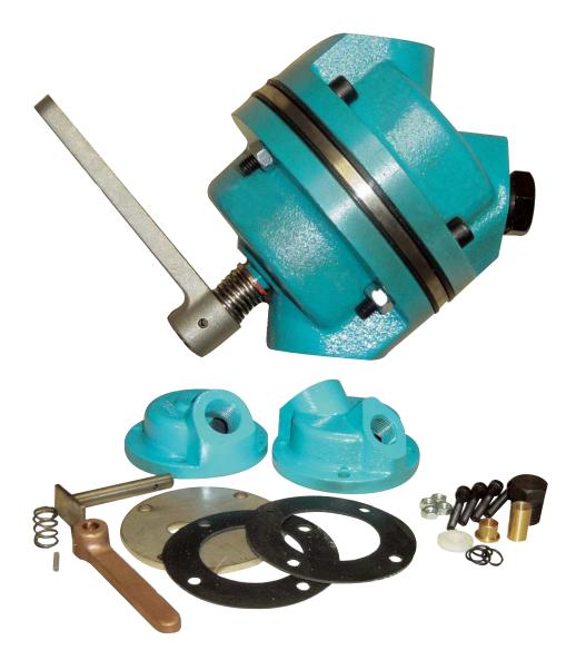
The metering plate is adjusted to expose the varying amounts of an orifice hole in the disc, thus varying the amount of abrasive flow to the blast nozzle.
