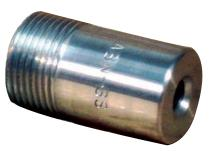
The ABN-S Series of nozzles are the same as the ATN-S, however feature boron inserts instead of tungsten carbide. Boron provides for a lighter nozzle, as well as a longer wear life.
